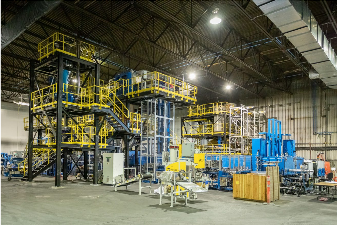
NMG's brand new 2,000-tpa coating module is being commissioned; production of CSPG expected by the end of Q3-2022.
