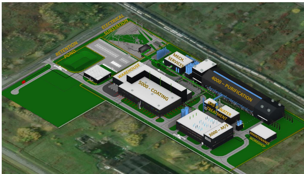
Figure 18-20: Proposed site plan for the Advanced Battery Material Plant in Bécancour
