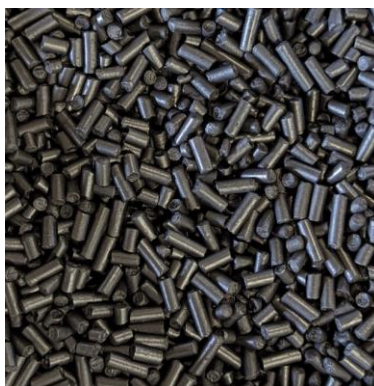
Figure 13-16: Granule of by-product classification coarse particle with activated starch binder
